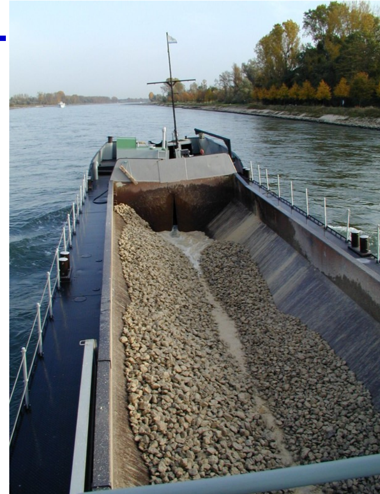
split barge downstream Iffezheim
