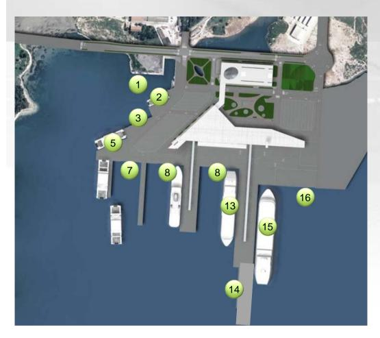
The marine facilities consist of twelve berths totalling 1 851 m in length with depths ranging from 5 m to 13 m, including:
