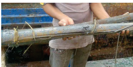
Bamboo extracted from Breakwater Dam Citra constructed in 1961 (Courtesy Toyo Construction)
