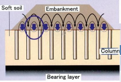
From the results of the joint study, we have establish new soft soil improvement concept as ALiCC method. The use of ALiCC technology has spread even to all in Japan because of its shorter construction time against the conventional PVD option. We have identified the shape of the arch effect between DM columns with simple formula.
