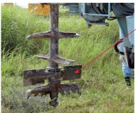
Free Blade is longer than other blade and free from rotation. So it can be fixed in the ground and assists the well mixing.
