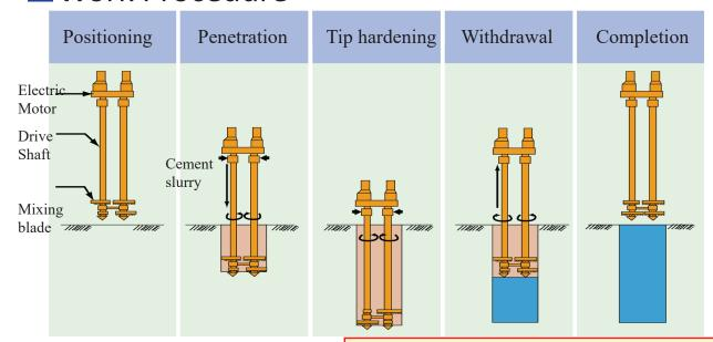
Diameter of mixing blade: 1.0 to 1.6 m
