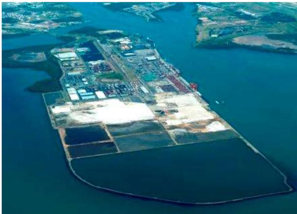
**Channel maintenance dredging materials** consisting of river muds capped with sand was used. The thickness of the fill was up to 9 m. The seabed compressible clay was over 30 m.
