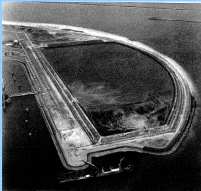
Fig. 5.14 : The "Parrot's Beak" is being filled with heavily polluted material. The jetty at the bottom of the photograph is for self-unloading hopper dredgers. (With kind permission of the Port of Rotterdam)
