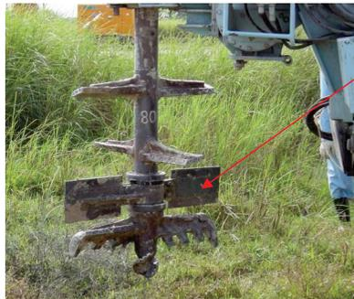
Free Blade is longer than other blade and free from rotation. So it can be fixed in the ground and assists the well mixing.
